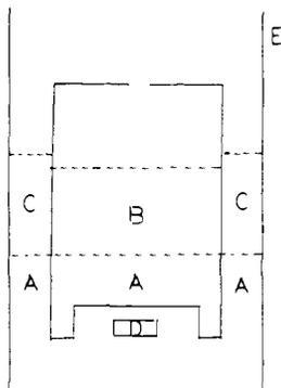
**Figure 1.** Apparatus used for transport studies. (A) Lower layer, 150 mL of 0.7 mM ionophore in  $\text{CH}_2\text{Cl}_2$ ; (B) inner layer, 40 mL of 0.05 or 0.0125 M KSCN in deionized, distilled water; (C) outer layer, 50 mL of 0.02 M  $\text{Fe}(\text{NO}_3)_3$  in 0.2 M aqueous  $\text{HNO}_3$ ; (D) stirring bar; (E) 600-mL beaker.
